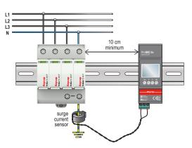
The ProSEC II+ is a surge counter with additional functionality. Besides counting the number of surges, it also logs the hour and date of each surge counted. This additional time and date logging function makes it possible to pinpoint the exact time of every surge and correlate it with equipment and power supply problems inside of a facility or structure.
